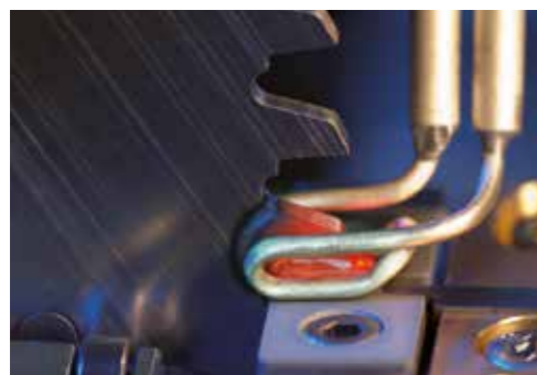
Fig. 12: Brazing of saw tips to a steel saw body
